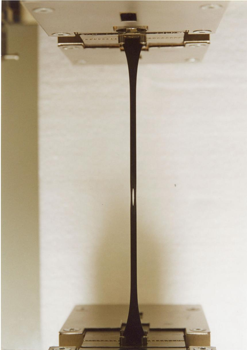
Fig.3: Tension test at a sample with a circular notch
