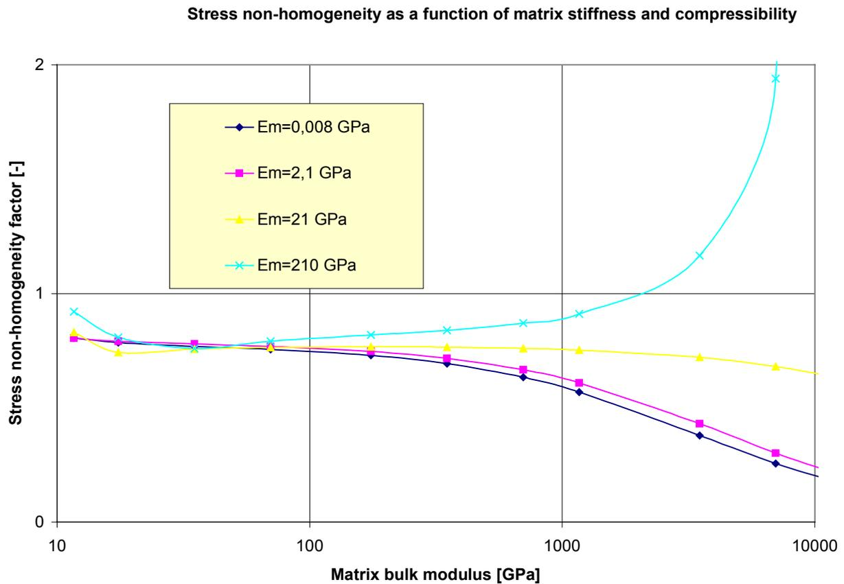
Fig.5: Stress non-homogeneity vs. matrix bulk modulus. Fibre elasticity modulus and fibre Poisson's ratio kept constant ( $E_f = 210$  GPa,  $\mu_f = 0,3$ ).
