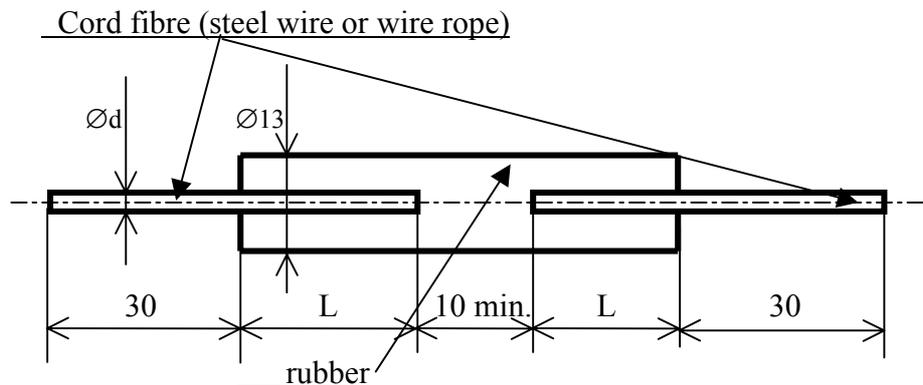
Fig. 1: Samples for measuring the rip-out force
