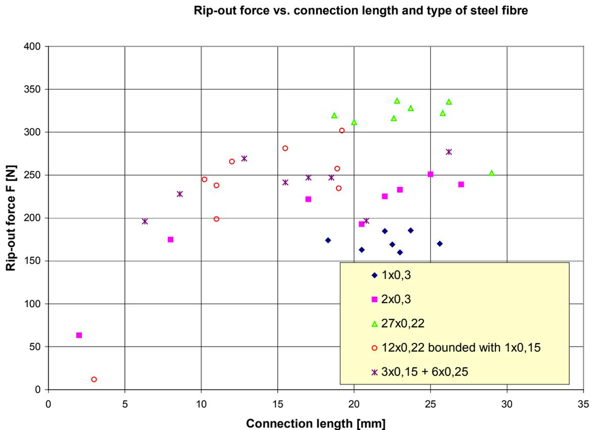
Fig. 2: Experimental results of adhesive forces measuring
