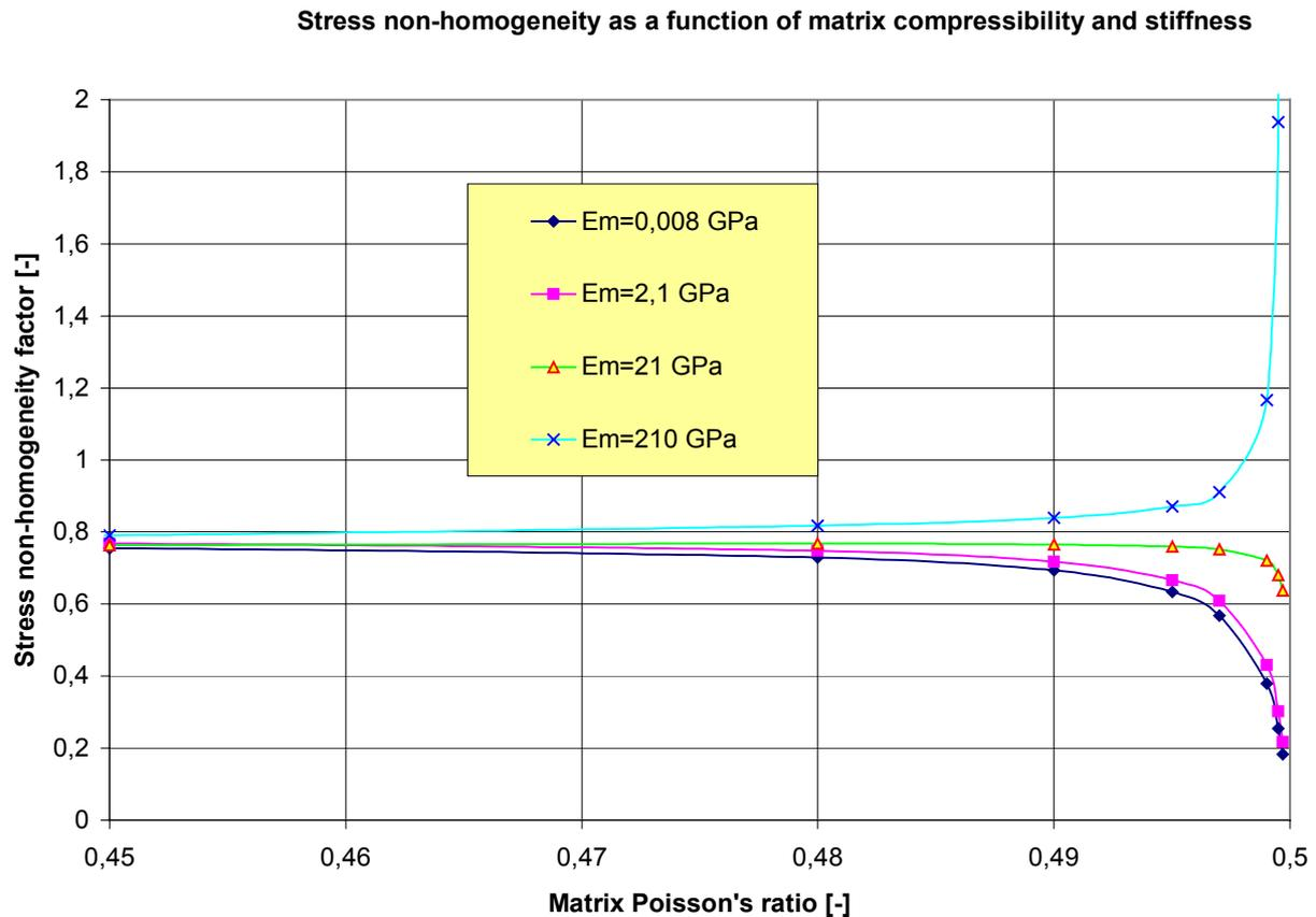
Fig.4: Stress non-homogeneity against matrix Poisson's ratio. Fibre elasticity modulus and fibre Poisson's ratio kept constant ( $E_f = 210$  GPa,  $\mu_f = 0,3$ ).
