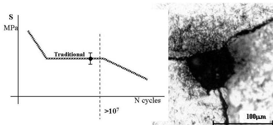
Fig.2. The oxide inclusion or crack site and its vicinity for a stress of 510MPa  $9.70 \times 10^7$  cycles.
