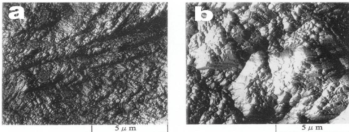
Fig.3. AFM image illustrating (a) Outside the process zone (b) At the process zone
