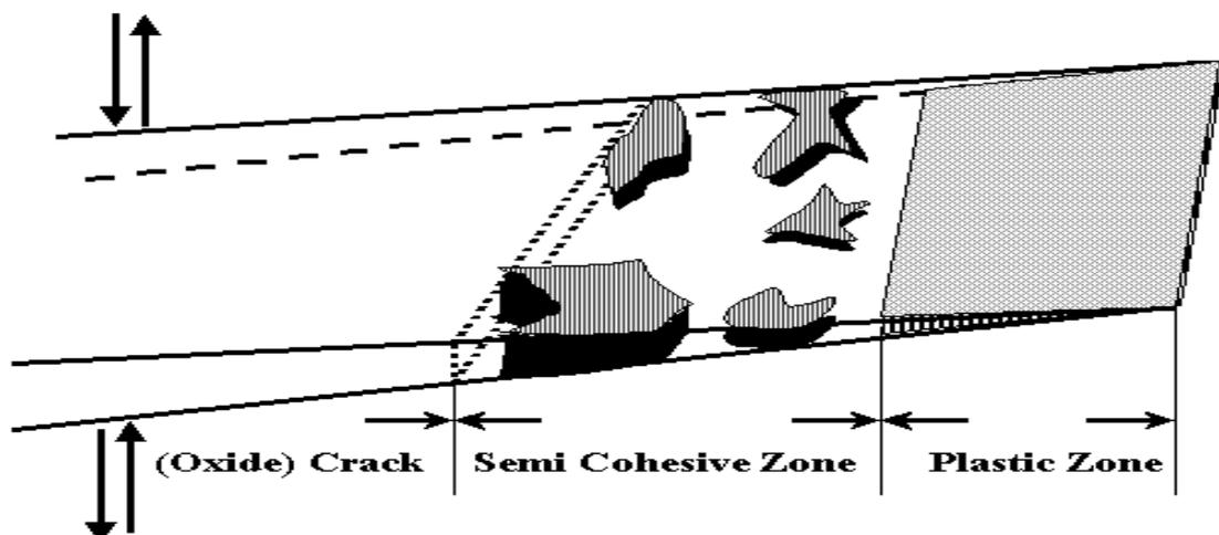
Fig.5. Schematic, semi cohesive zone providing traction forces caused by the ligaments
