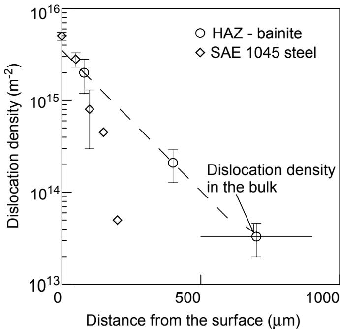
Fig. 4. Dislocation density vs. the depth below the surface in HAZ of the weld.
