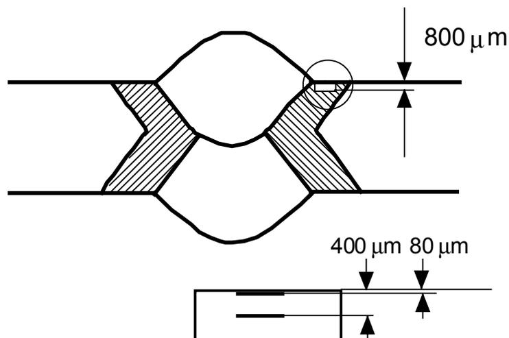
Fig. 1. Central part of the welded specimen and the location of the foil in HAZ. From the welded sheet a specimen whose width was 15 mm was cut. Figure 1 shows schematically the central part of the specimen with the weld and HAZ on both sides. The
