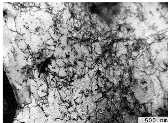
Fig. 4. Dislocation structure in HAZ in the depth 400  $\mu\text{m}$  below the surface after shot peening.
