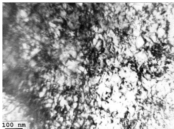
Fig. 3. Dislocation structure in HAZ in the depth 80  $\mu\text{m}$  below the surface after shot peening.
