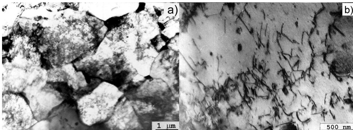
Fig. 2. Dislocation structure in HAZ in as-welded state.
