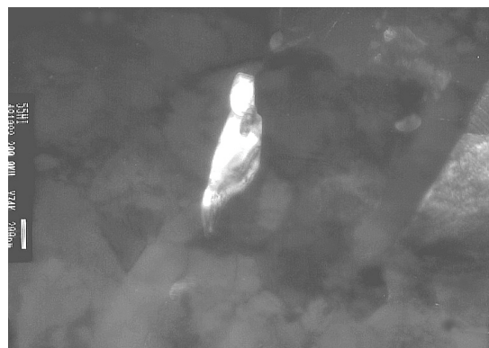
Figure 23 Dark field image of an inter-lath two-component carbide: M_{23}C_6 + M_6C in sample 580°C /5000h
