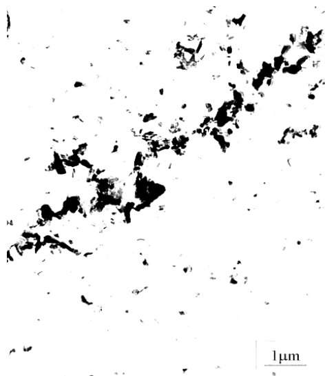
Fig. 3 Precipitates along prior austenite grain boundary, HT: Q + 690
