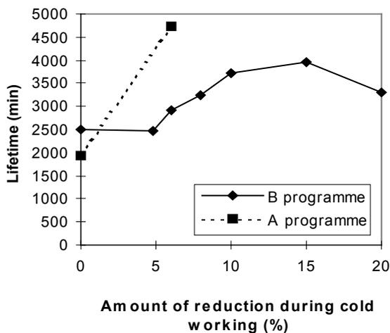
Fig. 2. The relationship between creep life and amount of reduction.
